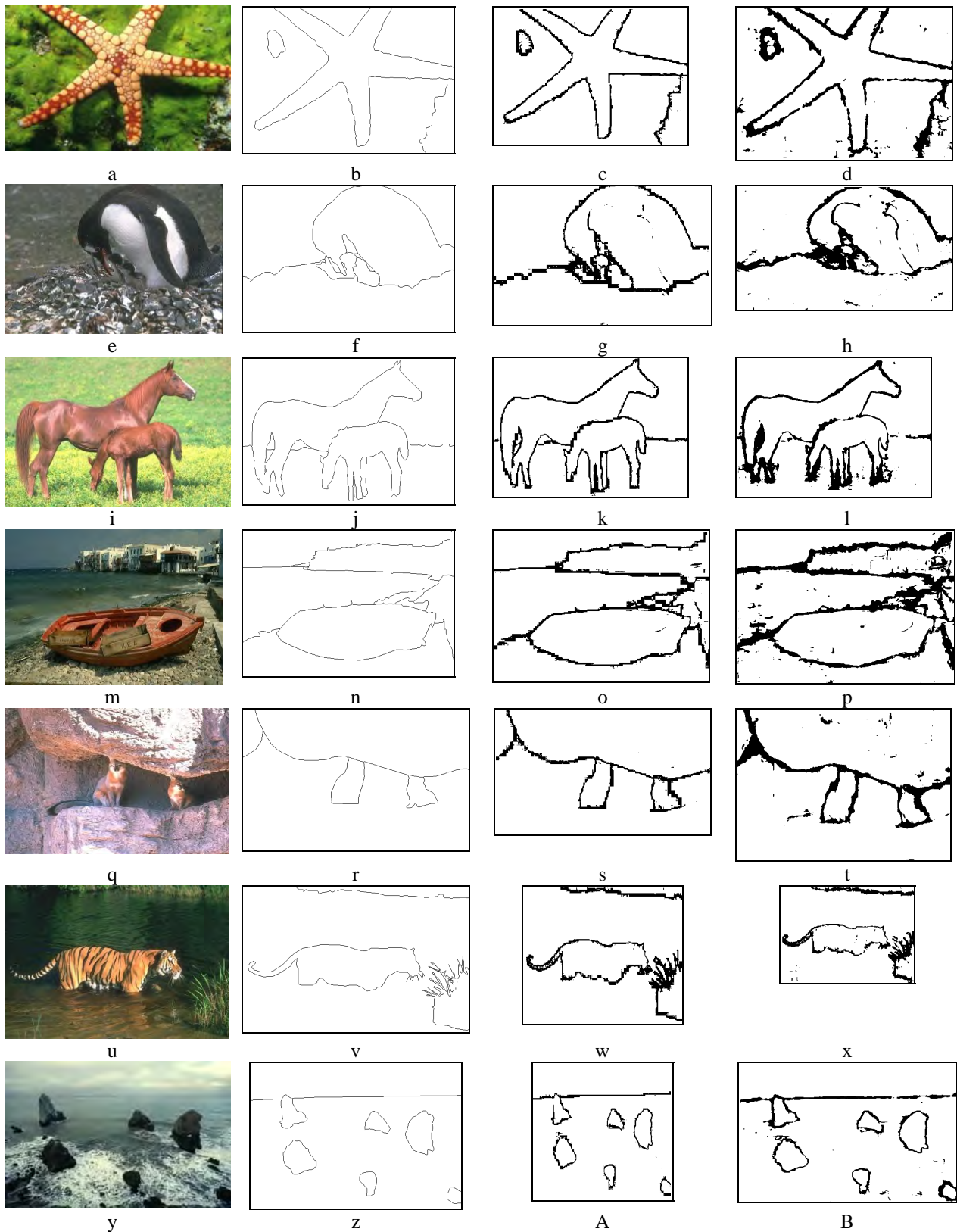
Figure 4 – The edge detection results by proposed RCF-ST network: a, e, i, m, q, u, y – the initial BSDS500 images; b, f, j, n, r, v, z – the ground-truth images; c, g, k, o, s, w, A – edge maps, obtained by RCF-ST network with transposed convolution; d, h, l, p, t, x, B – edge maps, obtained by RCF-ST network with interpolation
